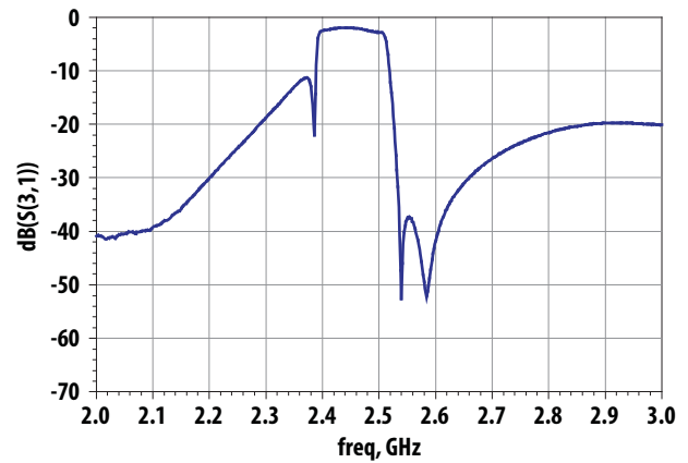
Figure 4. RX Path 2 – 3 GHz Frequency Response
